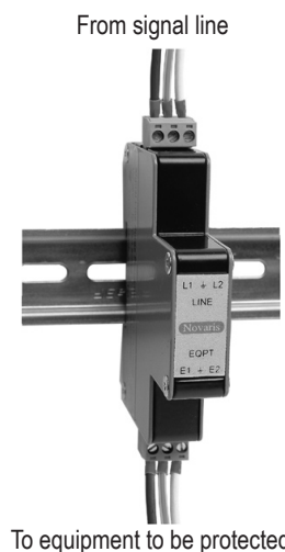
Figure 3: Signal line protectors are connected in series
