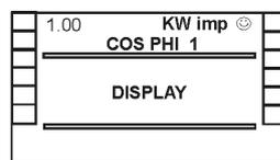
**Cos φ, valid Target cos φ (1 or 2):** Showing of power-factor and of the active target power factor (e.g. tariff switching with digital input).
