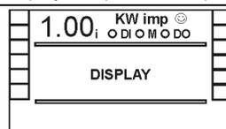
**Cos φ, DI, M, DO:** Display of power factor and status of inputs and outputs (○=inactive, ●=active)
