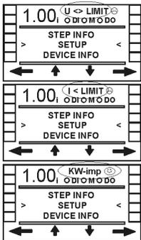
If the controller remains in this setup status for more than 5 sec use the flowchart above to check the VT ratio the nominal voltage and the connection of the voltage measurement.
